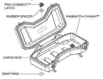
3. Lift the lever on each latch to unlock them. Place the cargo box onto the front rack of the ATV. Line up each latch with its corresponding hole in the rack then push each latch into its hole.
