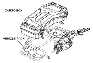
4. Secure the cargo box to the vehicle by pressing down each Honda Pro-Connect™ latch lever.
